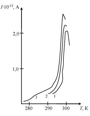
Figure 1 – Illustration of thermal cleaning of the TSC light emitted diode peak based on *GaAlAs* at a heating rate of  $\beta = 0,25$  K/s
