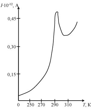
Figure 2 – Curve of the TSC current of a nondegraded LED at a heating rate of  $\beta = 0,112$  K/s
