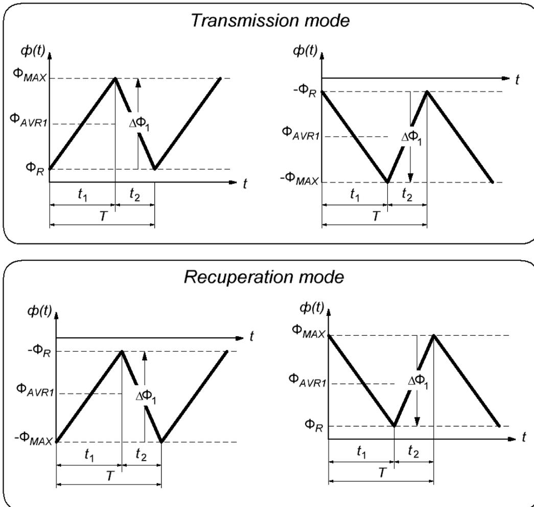
Figure 5 – Inductor core magnetic flux at the maximum power mode
