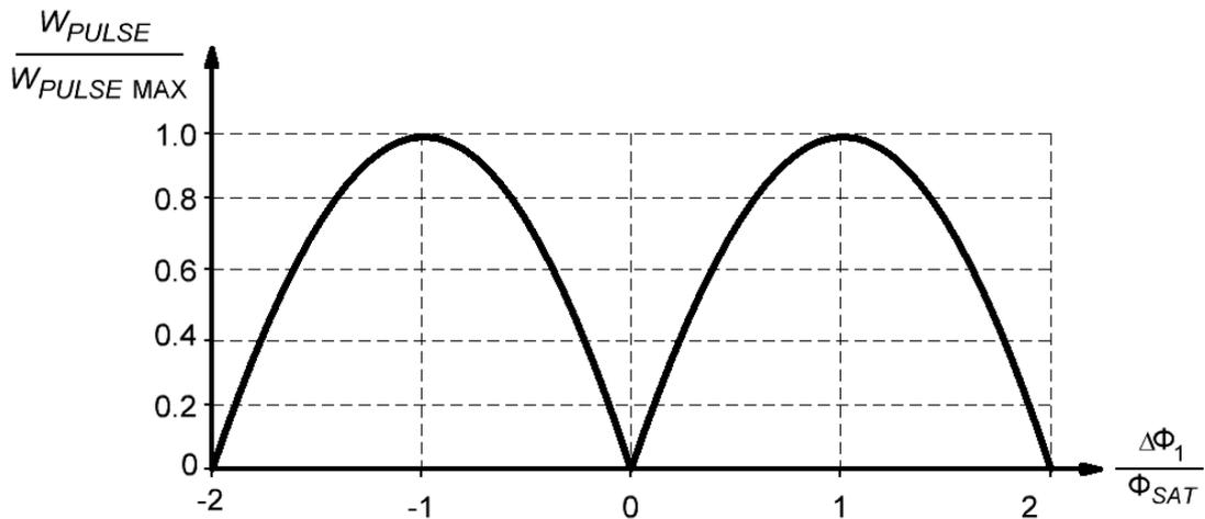
Figure 4 – Dependence of the quantity of energy  $W_{PULSE}$  on the value of magnetic flux change  $\Delta\Phi_1$
