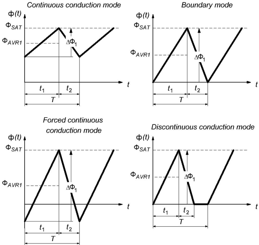
Figure 3 – Magnetic flux of the inductor core  $\phi(t)$  in various operating modes
