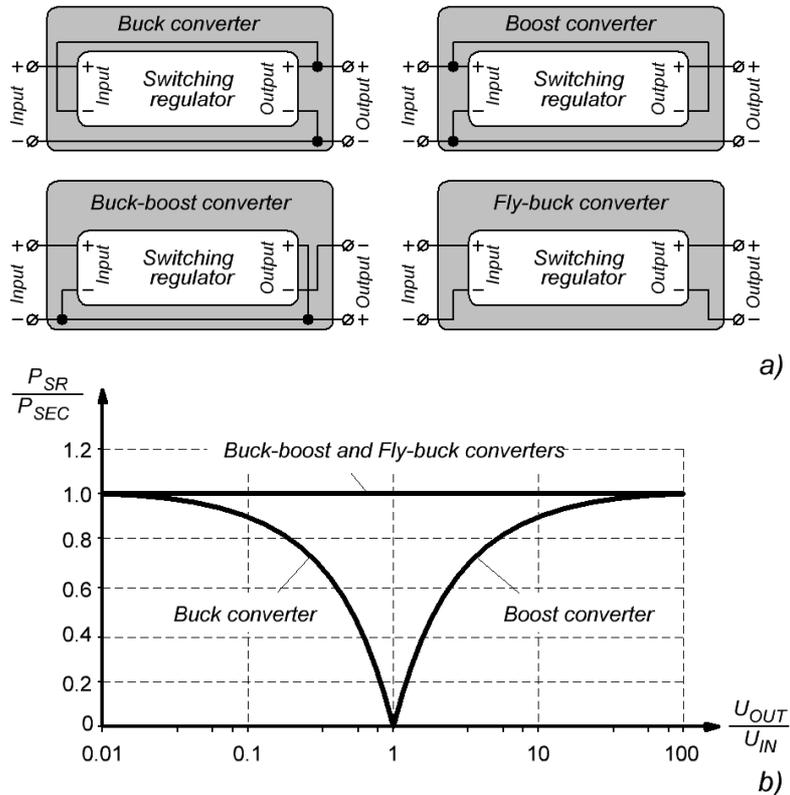
Figure 1 – The block diagrams of the most popular SECs a) and the dependence of their SR's relative power on the ratio of the SEC's input and output voltages b)
