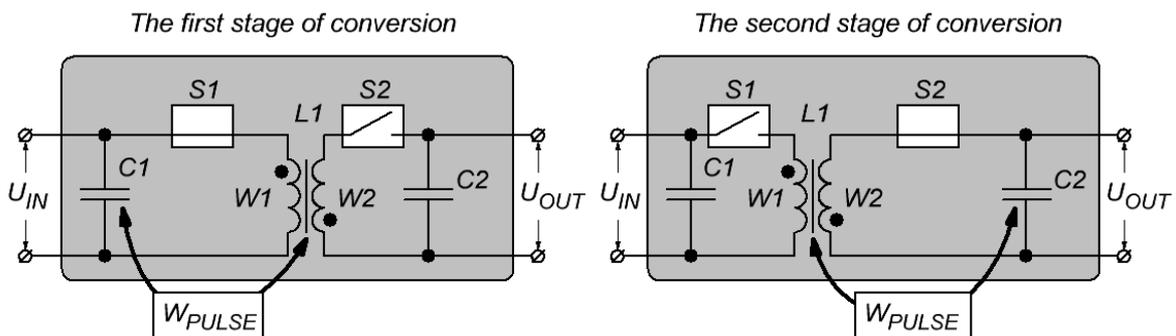
Figure 2 – The principle of switching conversion
