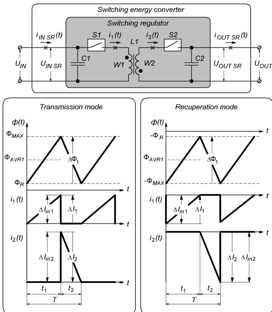
Figure 6 – SR's electrical processes at the boundary operation mode
