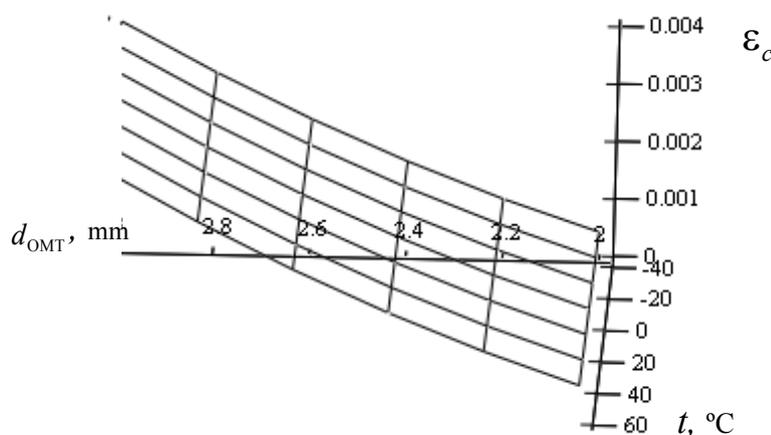
Figure 3 – Temperature dependence of relative elongation of the OC at different diameters of OMT
