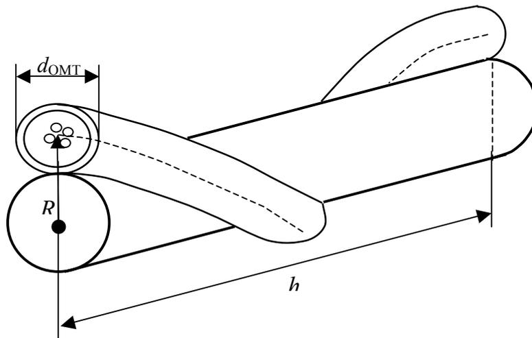
Figure 2 – Spiral stacking of the optical module tube around the CSE
