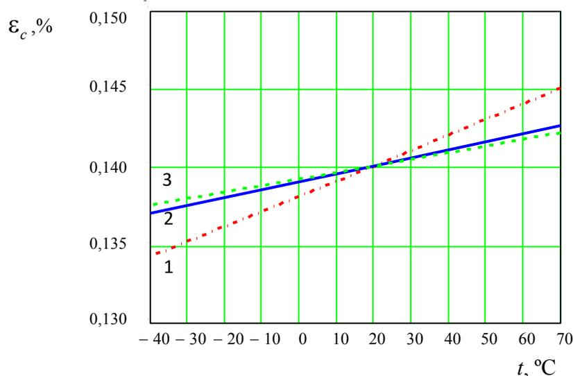
Figure 4 – Temperature dependence of relative elongation of OC for various materials of OMT: 1 – polybutylene terephthalate; 2 – polyamide; 3 – polycarbonate
