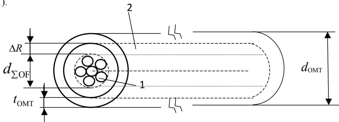
Figure 1 – Bunch of optical fibers, freely enclosed in the optical module tube:
