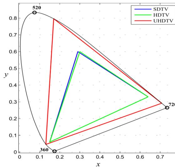
Figure 1 – Color primaries triangle of SDTV, HDTV and UHDTV systems presented on CIE-31 chromaticity diagram  $x, y$  coordinates plane
