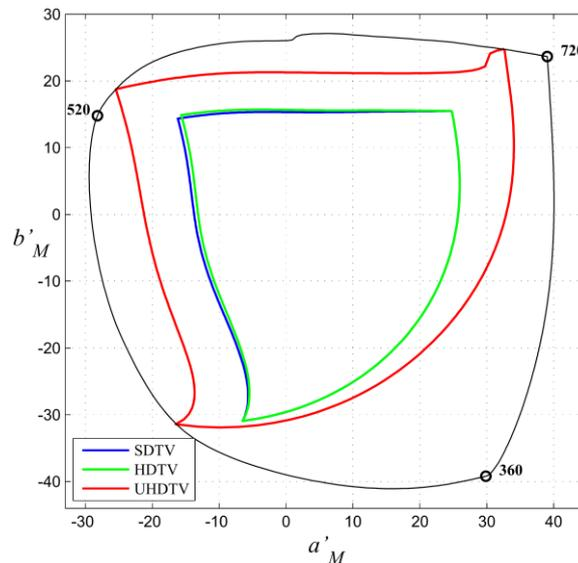
Figure 2 – Projections of color primaries triangle of SDTV, HDTV and UHDTV systems presented on the plane of coordinates of red-green ( $a'_M$ ) and yellow-blue ( $b'_M$ ) of uniform CAM-USC color space
