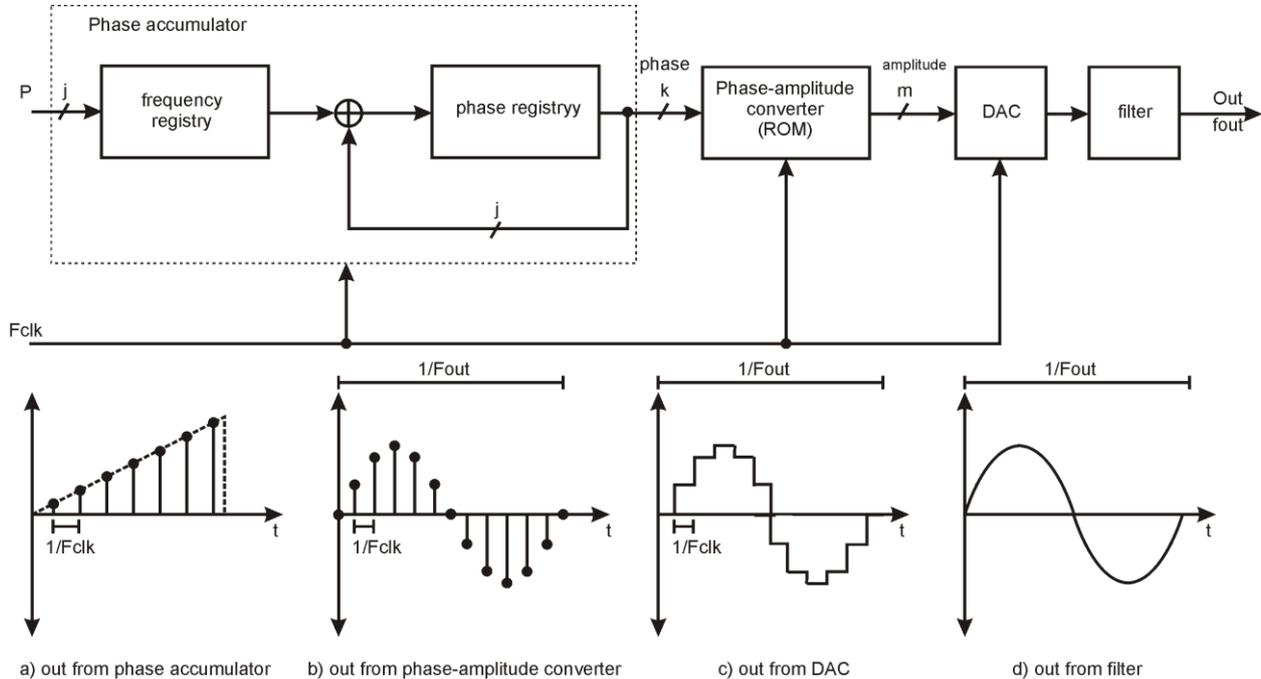
Figure 1 – Block diagram DDS and signal conversion rates.
