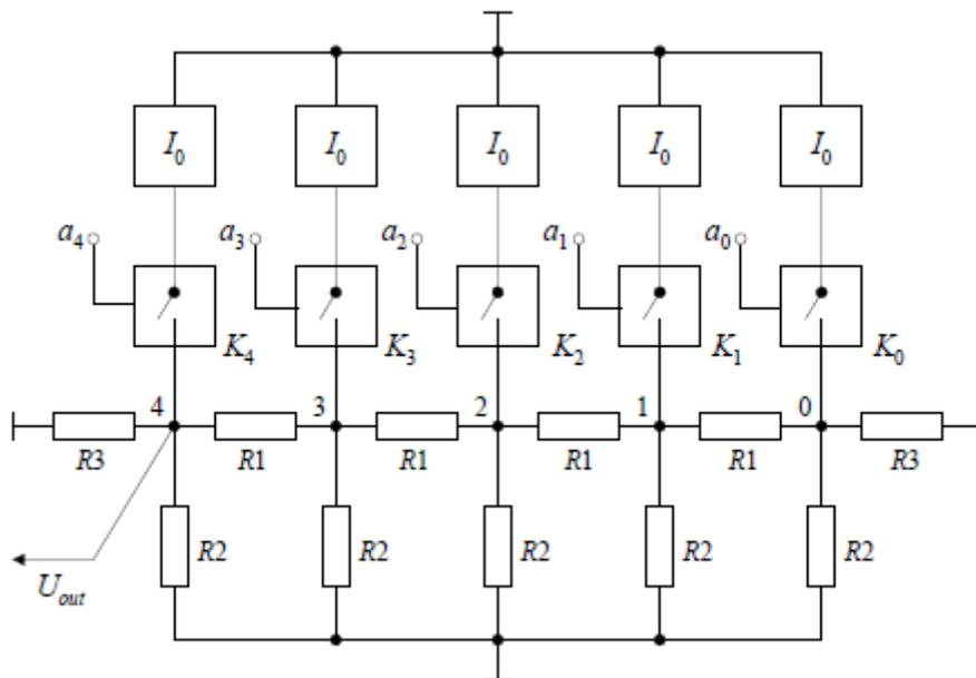
Figure 2 – Digital-to-Analog Converter Fibonacci
