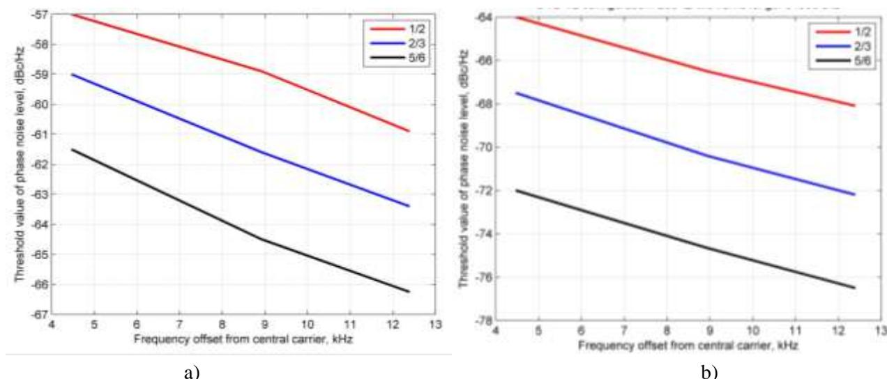
Figure 6 - Dependence of threshold level of phase noise from frequency offset for 16-QAM (a) and 256-QAM (b) modulations in DVB-T2 system
