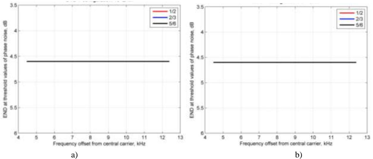
Figure 16 - Dependence of equivalent noise degradation value from frequency offset at presence of phase noise for 16-QAM (a) and 64-QAM (b) in DVB-T system
