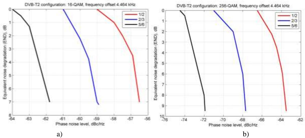
Figure 8 - Dependence of equivalent noise degradation value from phase noise level for 16-QAM (a) and 256-QAM (b) in DVB-T2 system
