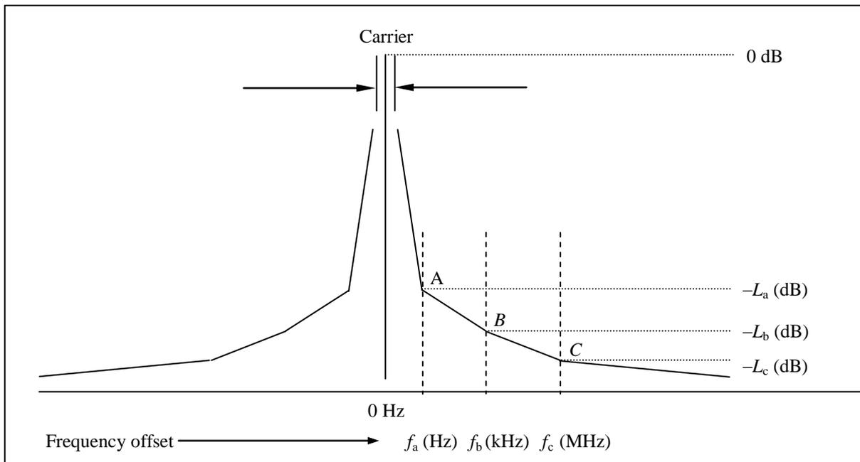
Figure 2 - Spectrum mask for CPE measurement
