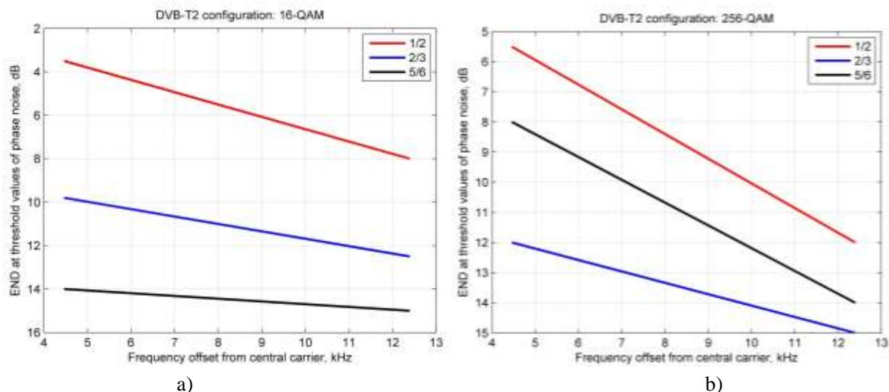
Figure 18 - Dependence of equivalent noise degradation value from frequency offset at presence of phase noise for 256-QAM in DVB-T2 system
