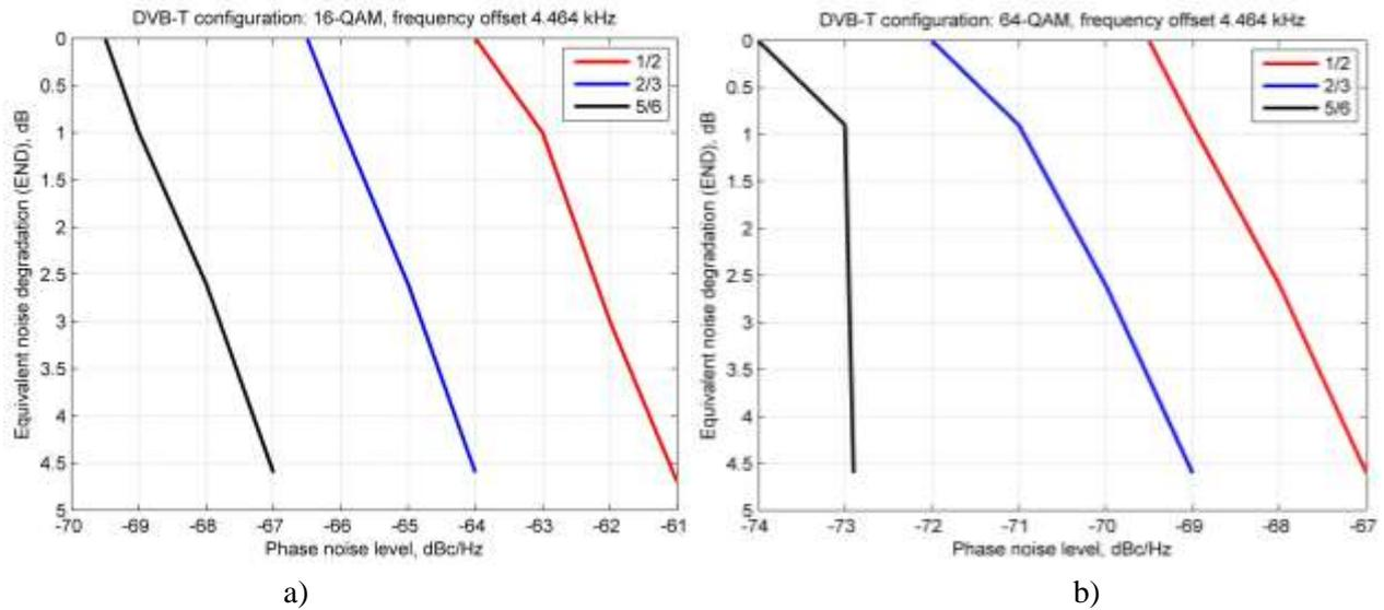
Figure 7 - Dependence of equivalent noise degradation value from phase noise level for 16-QAM (a) and 64-QAM (b) in DVB-T system
