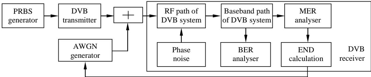
Figure 1 - Test set-up for estimation of phase noise impact on DVB-T and DVB-T2 system performance
