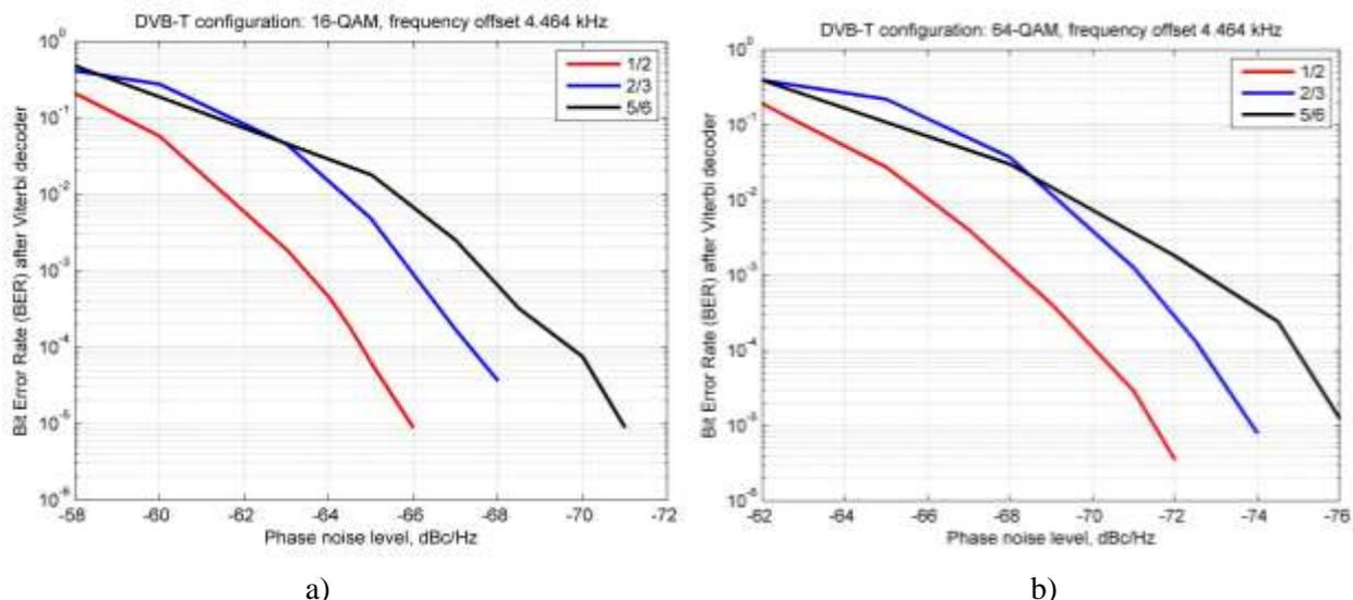
Figure 3 - Dependence of BER after Viterbi decoder from phase noise level in DVB-T system for 16-QAM (a) and 64-QAM (b) modulations and 4.464 kHz frequency offset
