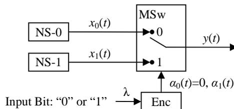
Figure 1 – Block-diagram of the transmitter of communication system with the help of the combined noise signals
