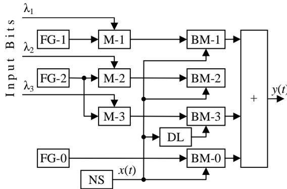
Figure 9 – "DISPERS" transmitter block diagram
