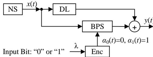
Figure 7 – Block diagram of Voronin system transmitter
