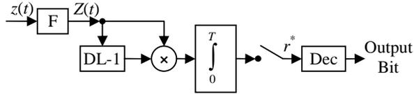
Figure 6 – Block diagram of the transmitter in the simplified Lange-Muller communication system
