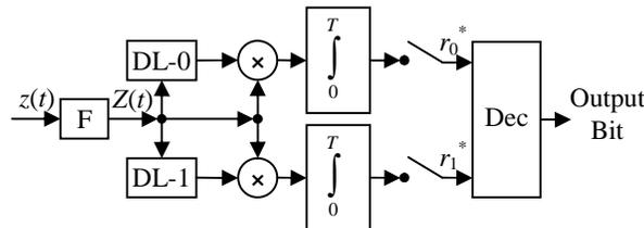
Figure 5 – CDNSK receiver block diagram
