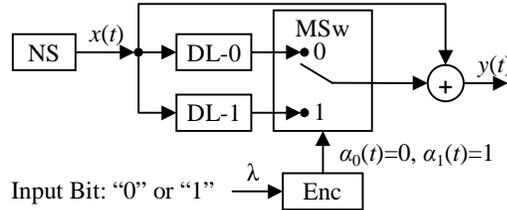
Figure 4 – CDNSK transmitter block diagram
