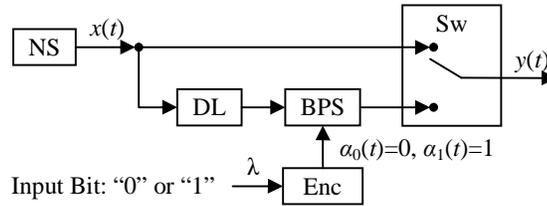
Figure 8 – DNSK transmitter block diagram
