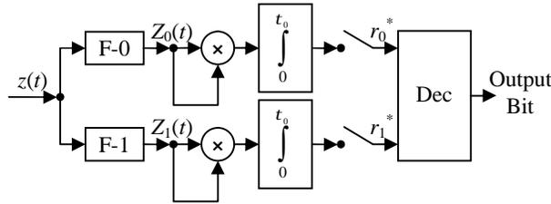
Figure 2 – Block diagram of a receiver for the two-component noise signal with a single change in the properties
