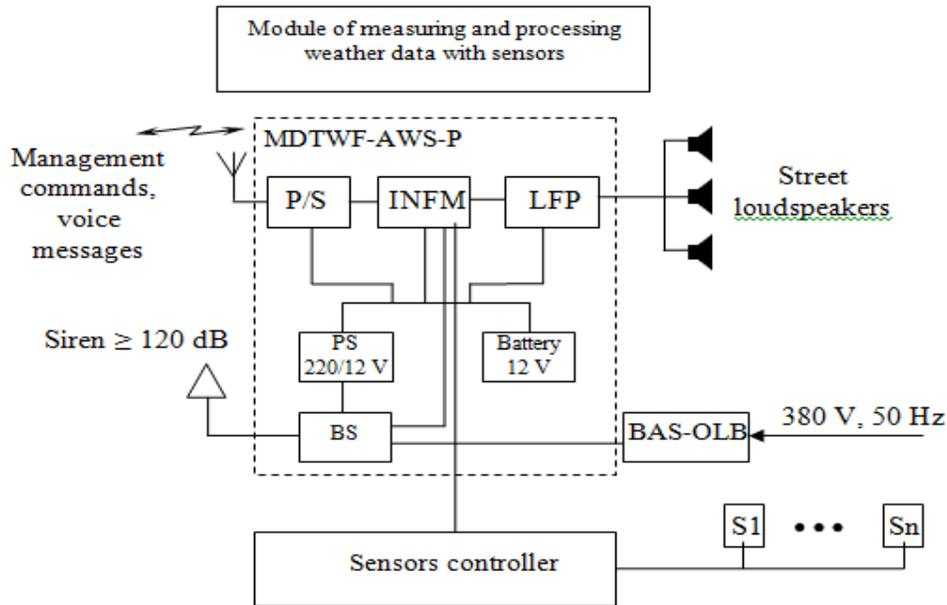
Figure 1 – Block diagram of radio-meteocomplex MCA-P
