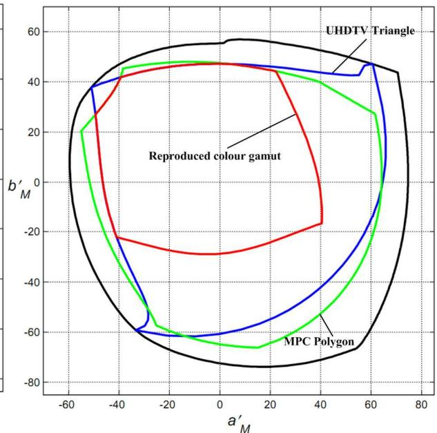
Figure 19 – Area of transmitted and reproduced chromaticities through light-to-light UHDTV system, when used six primary colors reproduction [6] for  $Y = 0.7$
