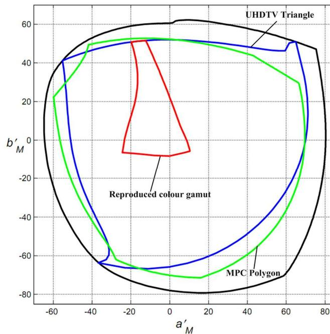
Figure 20 – Area of transmitted and reproduced chromaticities through light-to-light UHDTV system, when used six primary colors reproduction [6] for  $Y = 0.9$
