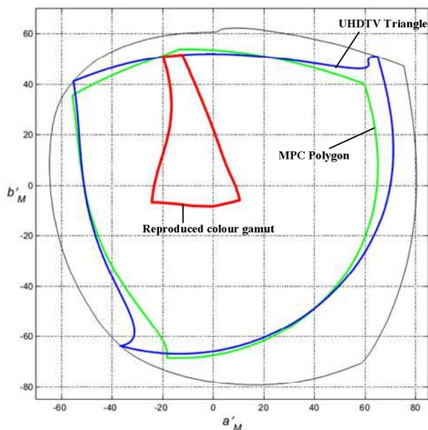
Figure 5 – Area of transmitted and reproduced chromaticities through light-to-light system, when used four colors reproduction with additional yellow for  $Y = 0.9$
