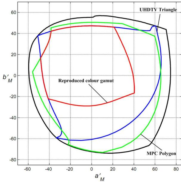
Figure 24 – Area of transmitted and reproduced chromaticities through light-to-light UHD TV system, when used six primary [7] colors reproduction for  $Y = 0.5$
