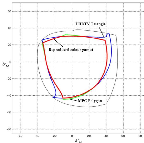
Figure 1 – Area of transmitted and reproduced chromaticities through light-to-light system, when used four colors reproduction with additional yellow for  $Y = 0.05$
