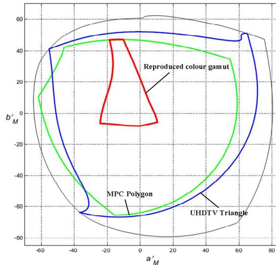
Figure 10 – Area of transmitted and reproduced chromaticities through light-to-light system, when used four colors reproduction with additional cyan for  $Y = 0.9$
