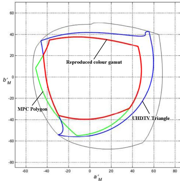
Figure 8 – Area of transmitted and reproduced chromaticities through light-to-light system, when used four colors reproduction with additional cyan for  $Y = 0.5$
