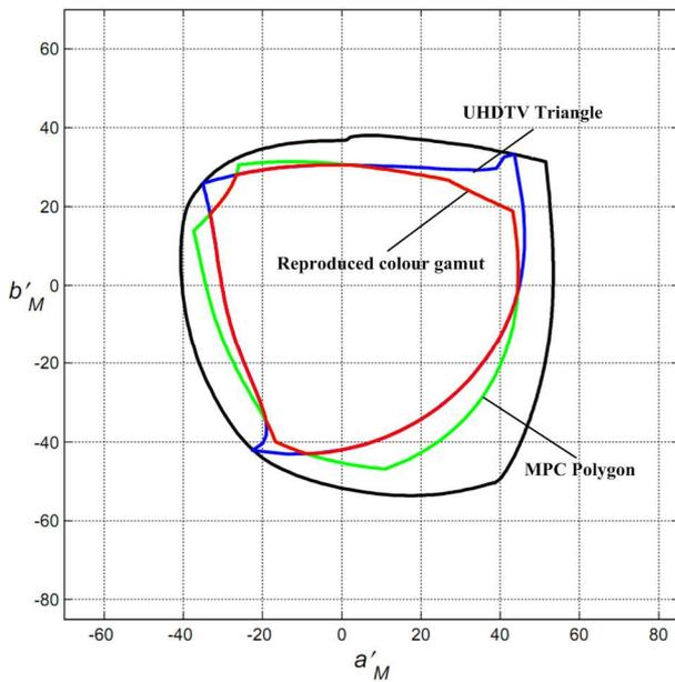
Figure 16 – Area of transmitted and reproduced chromaticities through light-to-light system, when used six primary colors reproduction [6] for  $Y = 0.05$
