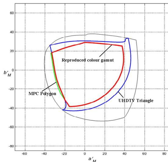
Figure 12 – Area of transmitted and reproduced chromaticities through light-to-light system, when used five primary colors reproduction with additional yellow and cyan for  $Y = 0.25$
