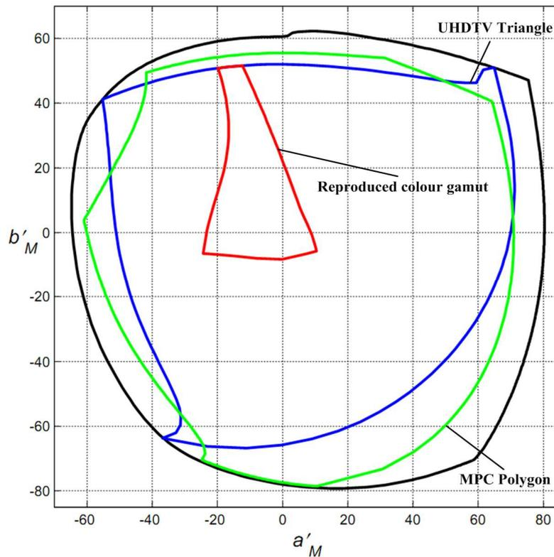
Figure 26 – Area of transmitted and reproduced chromaticities through light-to-light UHD TV system, when used six primary [7] colors reproduction for  $Y = 0.9$
