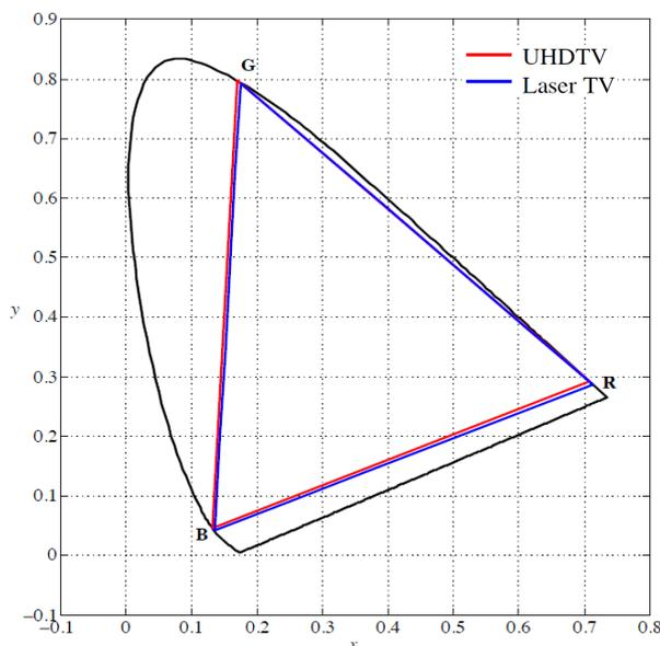
Figure 1 – CIE  $x,y$  chromaticity diagram of the laser TV system
