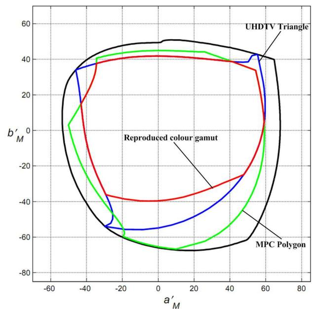
Figure 23 – Area of transmitted and reproduced chromaticities through light-to-light UHDTV system, when used six primary [7] colors reproduction for  $Y = 0.25$
