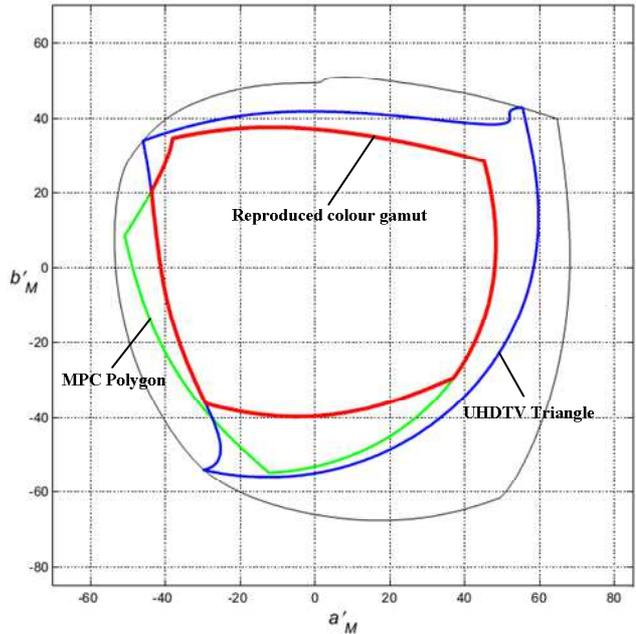
Figure 7 – Area of transmitted and reproduced chromaticities through light-to-light system, when used four colors reproduction with additional cyan for  $Y = 0.25$
