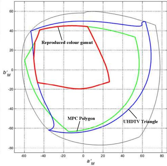
Figure 9 – Area of transmitted and reproduced chromaticities through light-to-light system, when used four colors reproduction with additional cyan for  $Y = 0.7$
