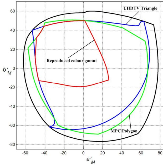
Figure 18 – Area of transmitted and reproduced chromaticities through light-to-light UHDTV system, when used six primary colors reproduction [6] for  $Y = 0.5$
