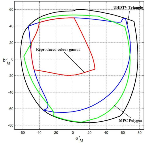
Figure 25 – Area of transmitted and reproduced chromaticities through light-to-light UHD TV system, when used six primary [7] colors reproduction for  $Y = 0.7$
