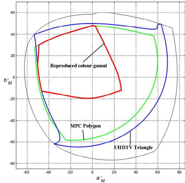
Figure 14 – Area of transmitted and reproduced chromaticities through light-to-light system, when used five primary colors reproduction with additional yellow and cyan for  $Y = 0.7$
