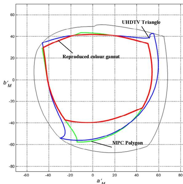
Figure 2 – Area of transmitted and reproduced chromaticities through light-to-light system, when used four colors reproduction with additional yellow for  $Y = 0.25$
