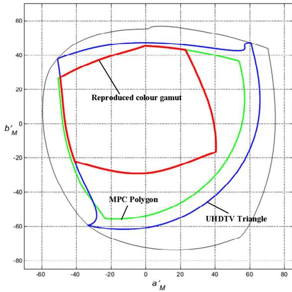
Figure 13 – Area of transmitted and reproduced chromaticities through light-to-light system, when used five primary colors reproduction with additional yellow and cyan for  $Y = 0.5$
