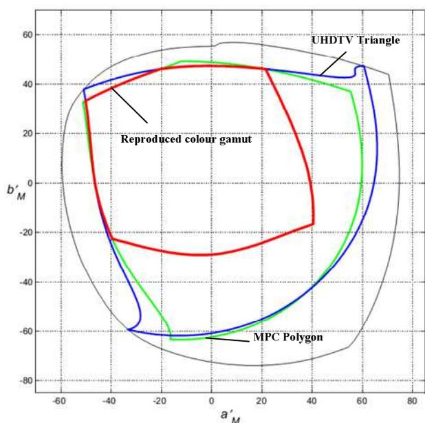
Figure 3 – Area of transmitted and reproduced chromaticities through light-to-light system, when used four colors reproduction with additional yellow for  $Y = 0.5$
