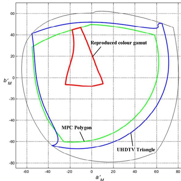
Figure 14 – Area of transmitted and reproduced chromaticities through light-to-light system, when used five primary colors reproduction with additional yellow and cyan for  $Y = 0.9$
