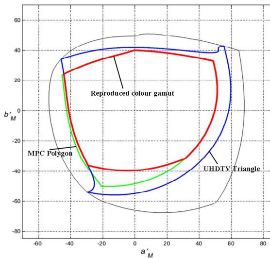
Figure 11 – Area of transmitted and reproduced chromaticities through light-to-light system, when used five primary colors reproduction with additional yellow and cyan for  $Y = 0.05$
