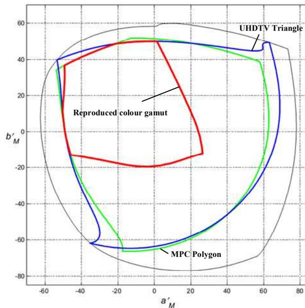
Figure 4 – Area of transmitted and reproduced chromaticities through light-to-light system, when used four colors reproduction with additional yellow for  $Y = 0.7$
