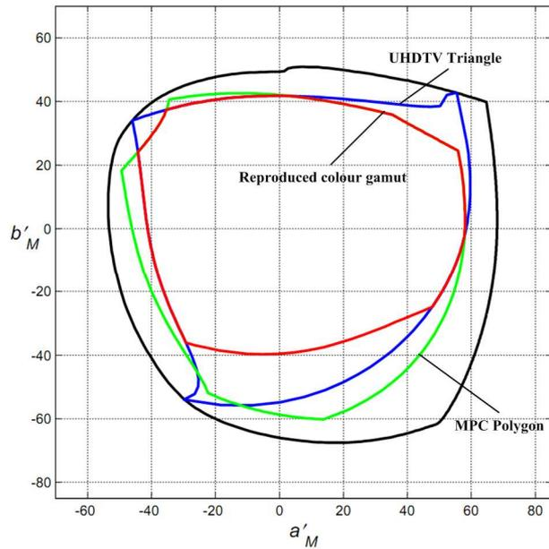
Figure 17 – Area of transmitted and reproduced chromaticities through light-to-light UHDTV system, when used six primary colors reproduction [6] for  $Y = 0.25$
