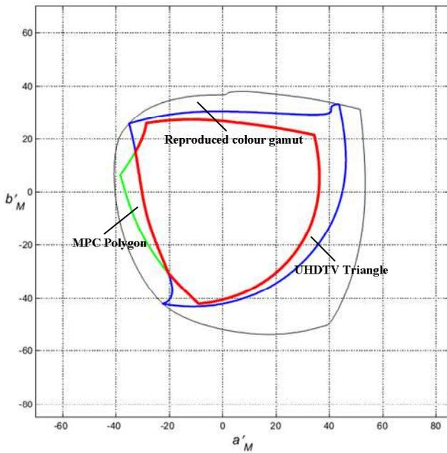
Figure 6 – Area of transmitted and reproduced chromaticities through light-to-light system, when used four colors reproduction with additional cyan for  $Y = 0.05$
