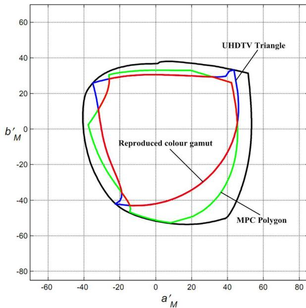
Figure 22 – Area of transmitted and reproduced chromaticities through light-to-light UHDTV system, when used six primary [7] colors reproduction for  $Y = 0.05$
