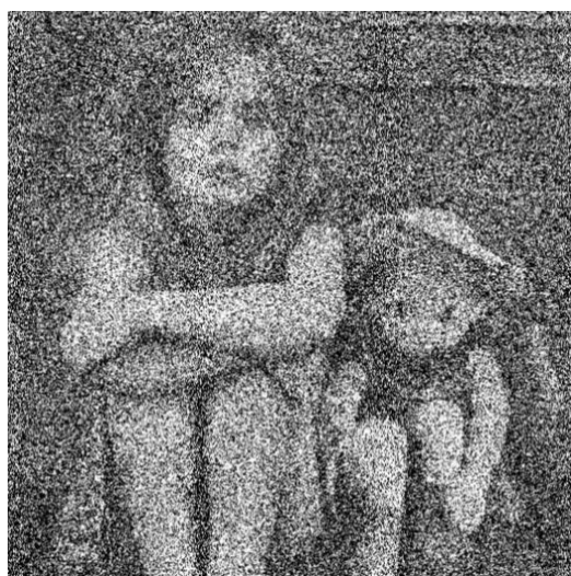
Fig. 5 The jamming influence on the image quality at the jamming-to-noise ratio equal to 36 dB
